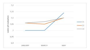
Fig. 3. pH variation of the waters of the three springs of the Oum Teboul region C1: Ain bergougaya, C2: source sigleb C3 source Siporex.
