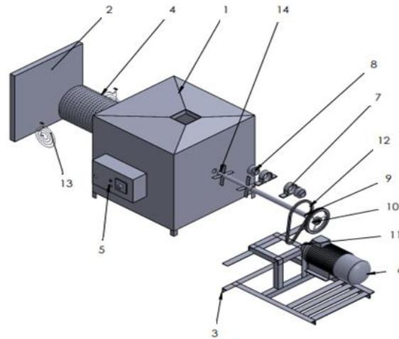
Fig. 1. The design cashew nut shelling machine:
