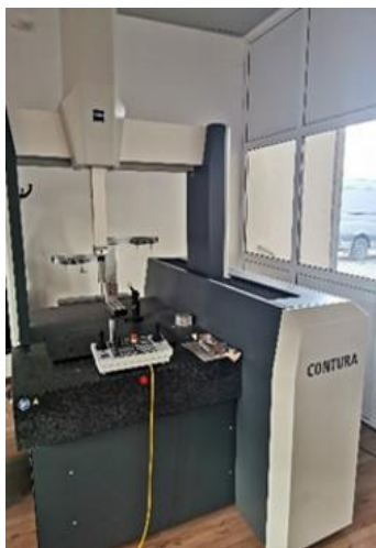
a. Zeiss Contura coordinate measuring machine [5]
