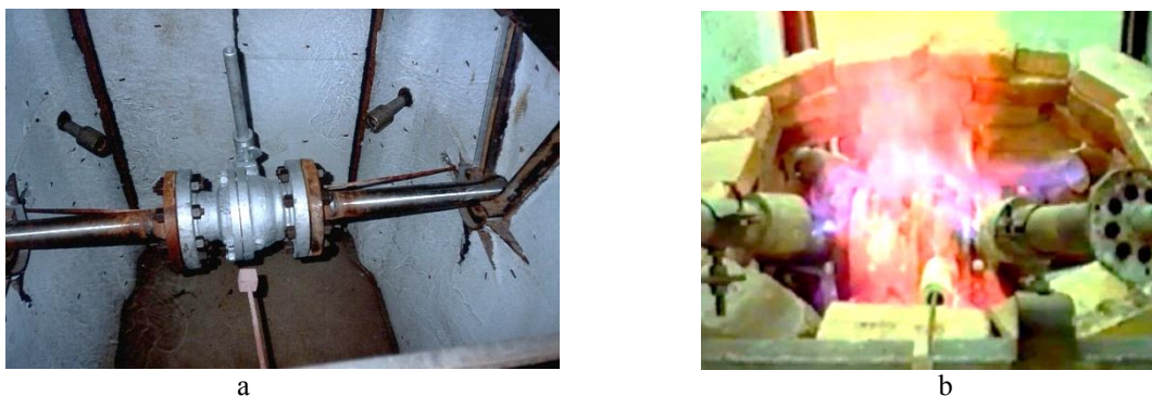
Fig. 3. The valve prototype attempted to fire: a. installation of temperature measurement sensors; b. burning the valve.
