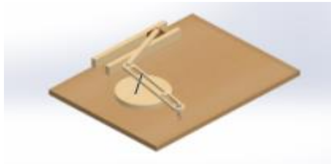
Fig. 2. Modelled Quick Return Mechanism using Solid work.
