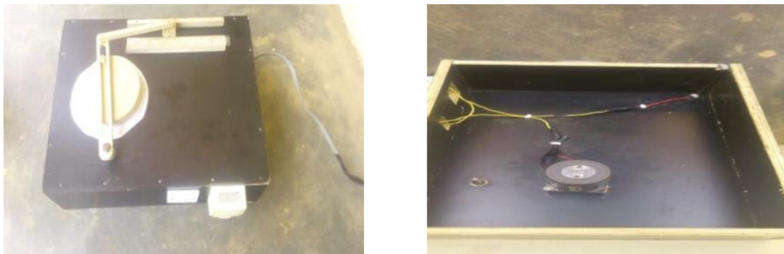
Fig. 3. Prototype Quick Return Mechanism constructed.
