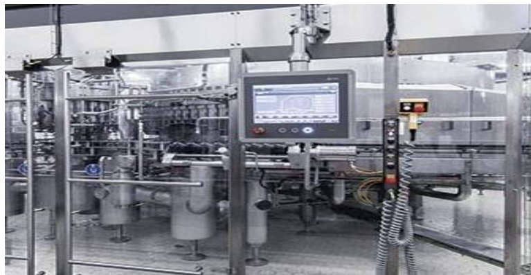
Fig. 2. Human Machine interface (HMI) for Filler System.
