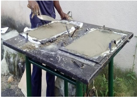
Fig. 1. Producing samples with Vibrating table.
