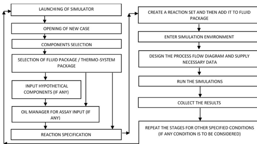
Fig. 3. Flow chart for simulating a process in Aspen HYSYS [11, 18].
