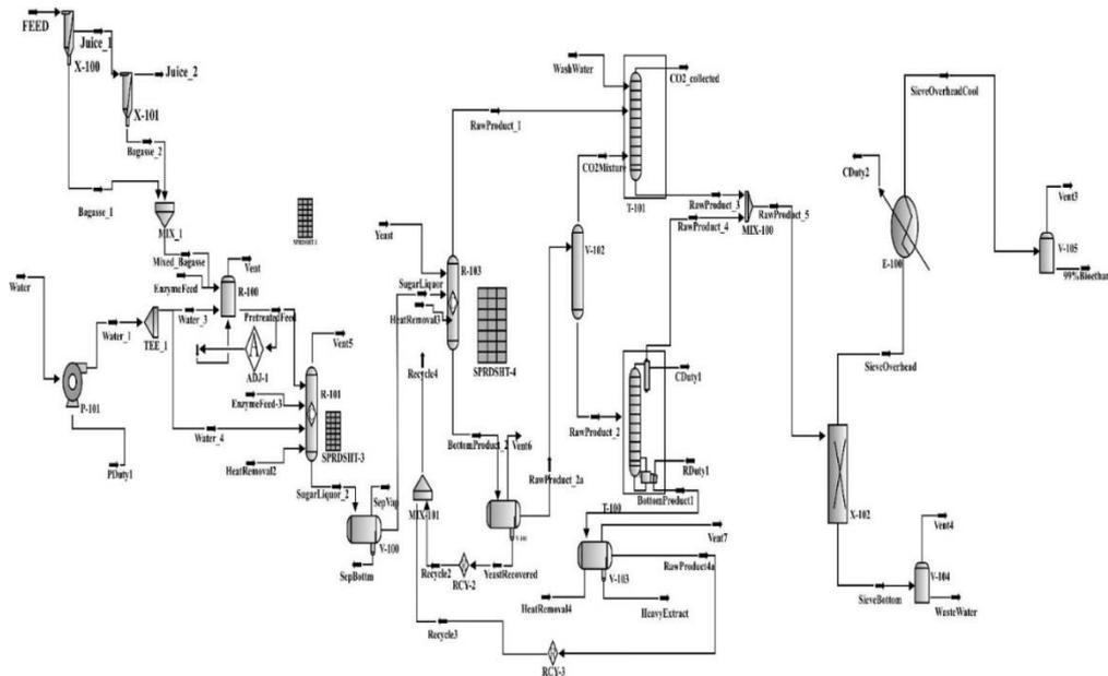
Fig. 4. PFD for bioethanol production from sorghum bagasse.
