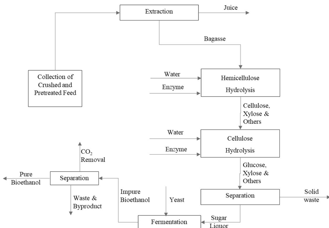
Fig. 2. Block flow diagram for the conversion of sorghum bagasse to bioethanol fuel.
