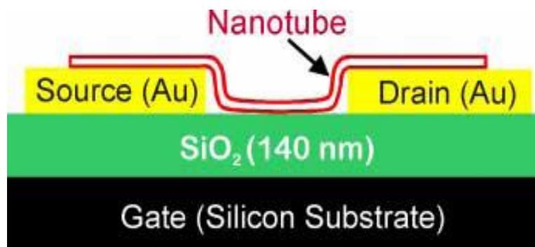
Fig. 1. Field-effect transistor based on a single 1.6 nm diameter carbon Nanotube [17].
