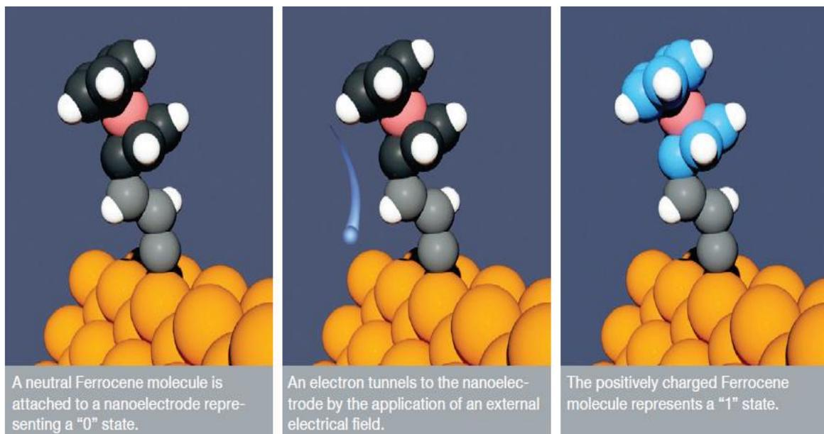
Fig. 3. Illustration of the alteration in state between the Ferrocene molecule from "0" to "1" state with the application of an external electrical field [25].
