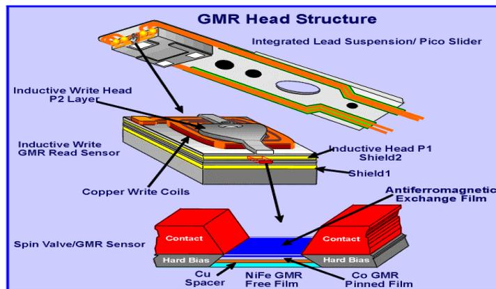
Fig. 2. Commercial IBM giant magnetoresistance read head [19].
