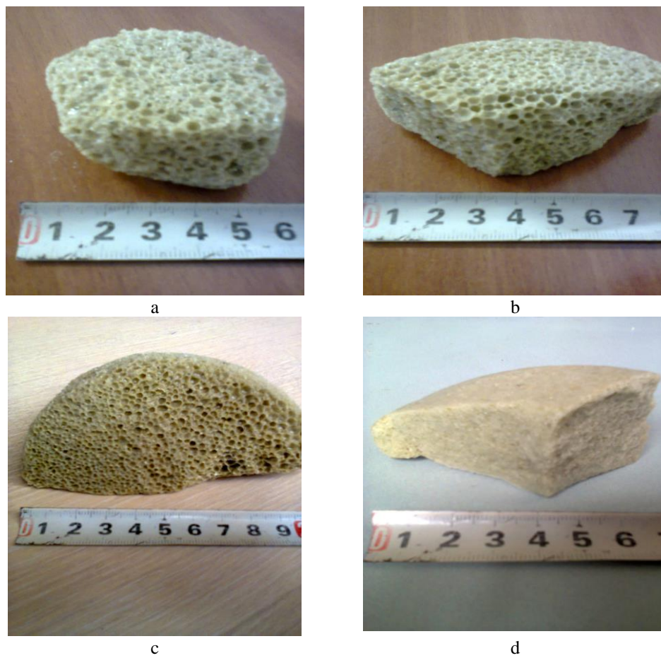
Fig. 2. Pictures of the foam glass gravel samples: a – sample 1; b – sample 2; c – sample 3; d – sample 4.
