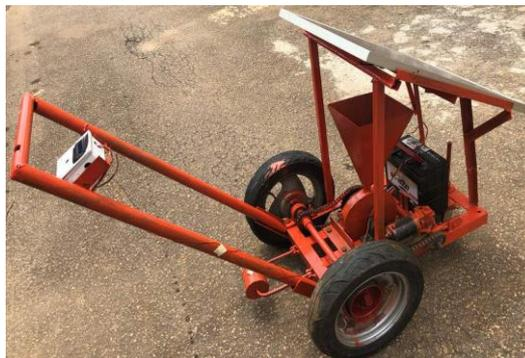
Fig. 7. Plate 3 - the fabricated planter.
