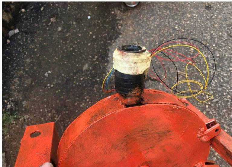
Fig. 5. Plate 1 - infrared light in seed delivery tube.
