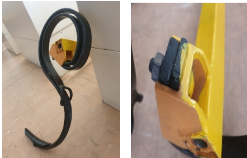
Fig.1. Working tool with elastic support.
