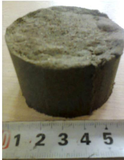
Fig. 2. Appearance image of the cold pressed powder mixture.
