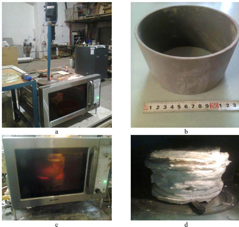
Fig. 1. The experimental microwave equipment: a - overall image of the equipment; b - ceramic tube; c - 0.8 kW-microwave oven; d - ceramic fiber thermal insulation.
