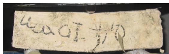
Fig. 6. Broken specimen showing a crack with the two pieces connected by the fibers.
