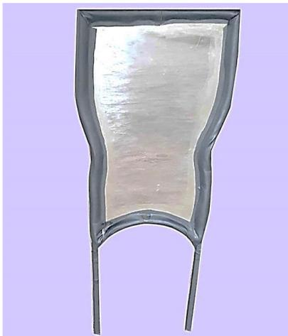
Fig. 8. Fabricated motorcycle protective isolation shield.
