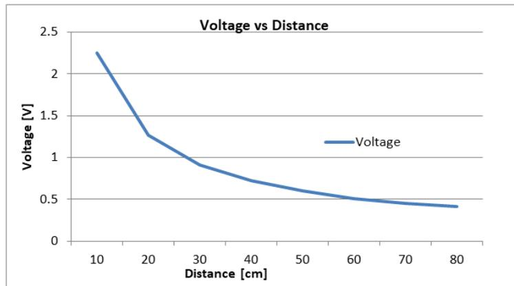
Fig. 6. The variation of the output voltage of the sensor depending on the set distance.
