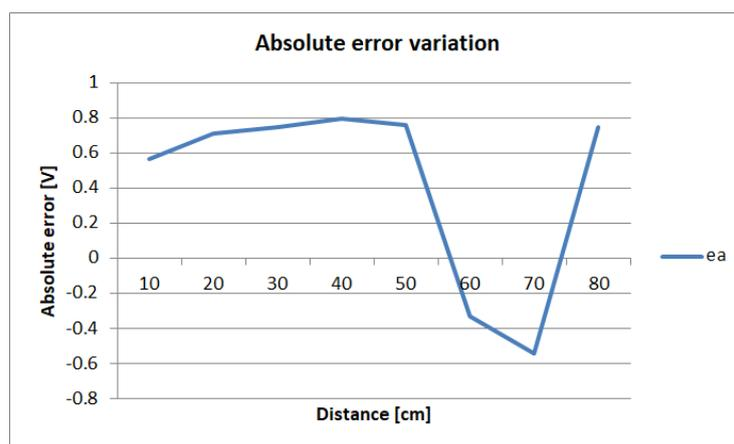
Fig. 7. The variation of the absolute error of the sensor depending on the set distance.
