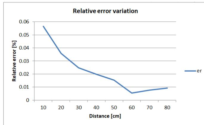
Fig. 8. The variation of the relative error of the sensor depending on the set distance.
