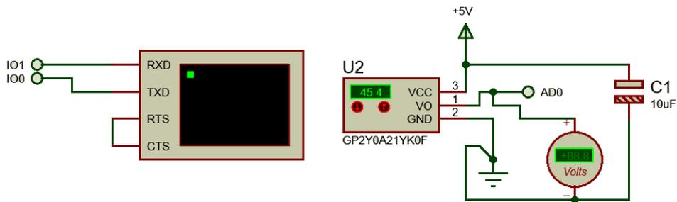
Fig. 4. Wiring diagram made in Proteus Professional 8.0 for simulating the GP2Y0A21YK0F proximity sensor.
