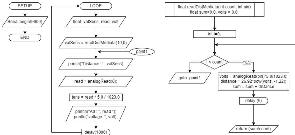
Fig. 5. Logic diagram of the program written in Arduino.
