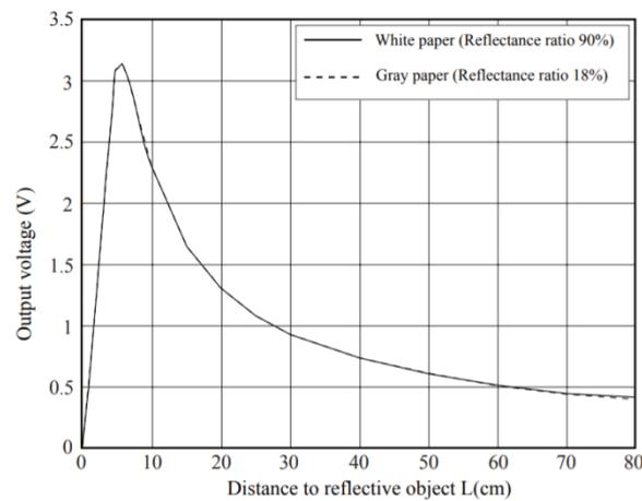
Fig. 3. Example of distance measuring characteristics (output).
