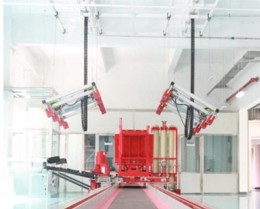
Fig. 5. Elevating device and the acceleration sledge.
