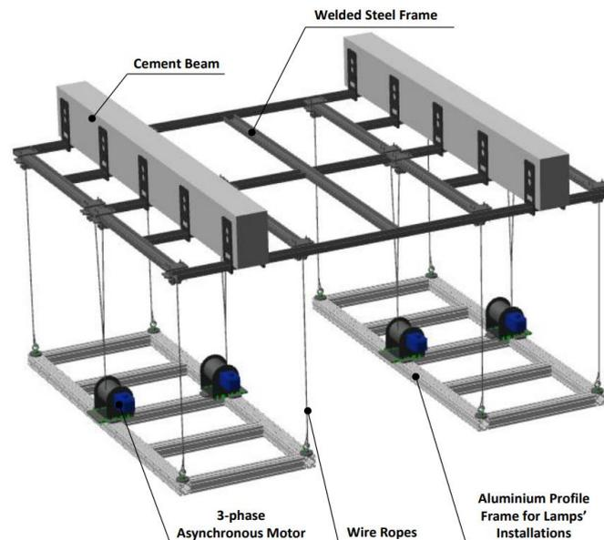
Fig. 3. 3-D display of the elevating device.
