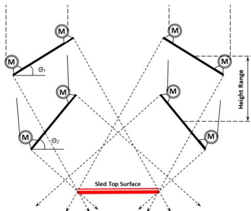
Fig. 9. Elevating limits of the elevating device in tests.
