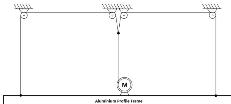
Fig. 4. Schematic diagram of elevating lamps.
