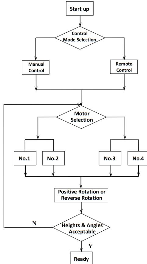
Fig. 2. Workflow of the elevating device.
