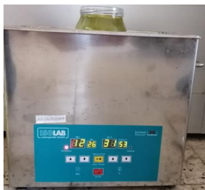
Fig. 1. Mixing of experimental fuels in an ultrasonic mixer.
