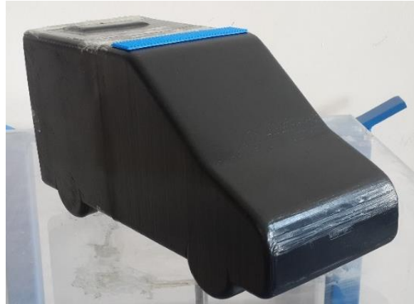
Fig. 3. Test model vehicle with non-smooth surface plate.
