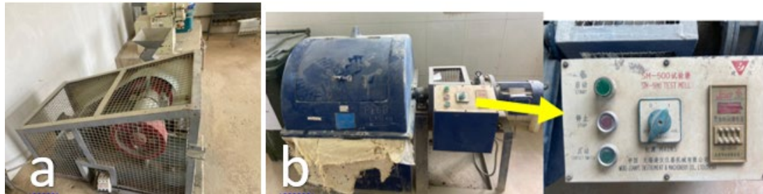
Fig. 6. Images with crusher machines: a) Crusher of the model ZBSX-92A Standard Sieve Shake; b) Ball mine crusher.
