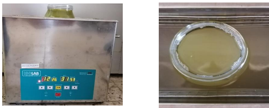
Fig. 2. Ultrasonic mixer and fuel with NPs.
