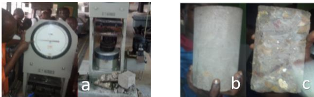
Fig. 7. (a) Crushing press for control mark; (b) test piece 110 x 220; (c) test piece after crushing.
