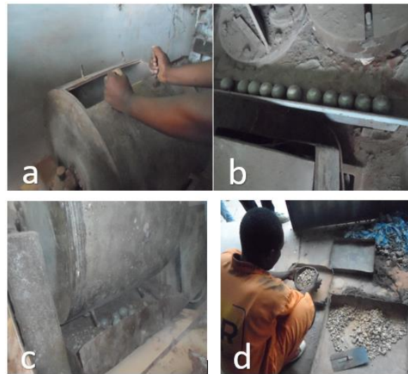
Fig. 5. (a) Los- Angeles Machine; (b) The 11 balls v; (c) Sampling the sandstone sample after test; (d) Sieving.
