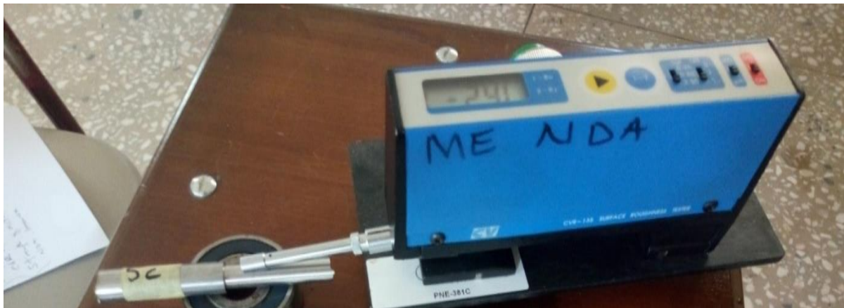
Fig. 3. A side view of the CRV 135 surface roughness tester used to measure the surface finishes of the produced steel samples.
