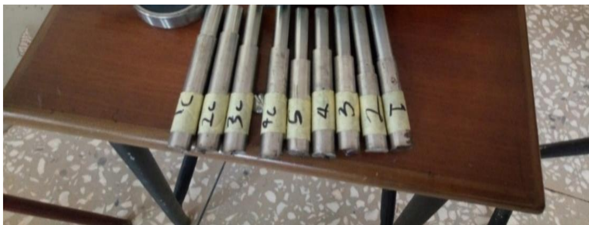
Fig. 2. Some of the produced medium-carbon steel samples at various turning conditions and their sequentially labelled identification marks.
