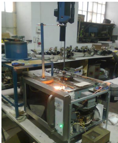
Fig. 1. The adapted 0.8 kW microwave oven.
