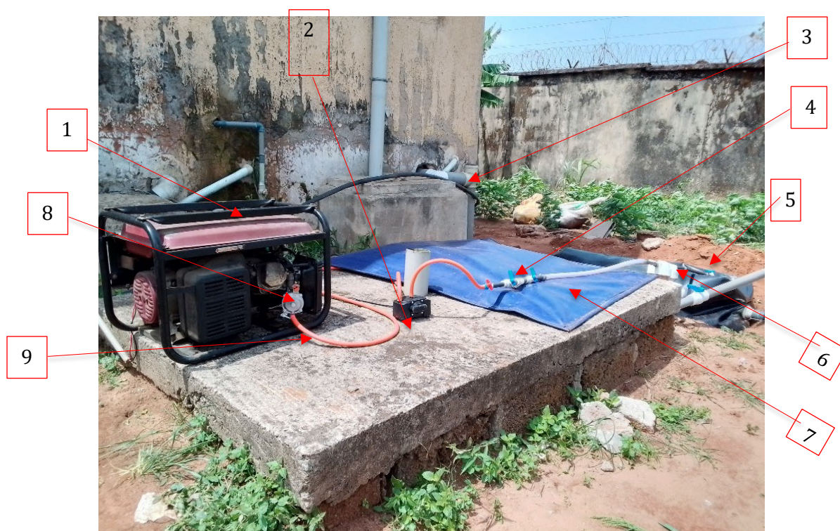
Fig. 2. Pictorial view of experimental configuration of human waste biogas production for power generation: 1- Modified generator; 2-Gas pressure regulator; 3-Inlet Valve; 4-Control Valve; 5-Bio-flex digester; 6-purification Unit; 7-gasholder; 8-hybrid Carburetor; 9-Gas host.
