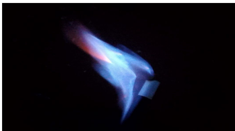
Fig. 4. Flammability test result of human waste biogas produce.
